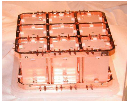
2 modules 9 detector 3 \times 3 \times 6 \text{ cm}^3 = 330 \text{ g} each 4 enriched: 2 \text{ }^{130}\text{Te} + 2 \text{ }^{128}\text{Te}
